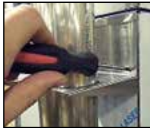
Tightening the Phillips screw
