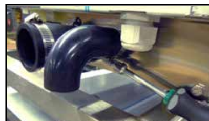
Install the spring clamp for the overflow elbow
